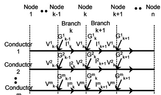
Fig. 1: Example of nodes and branches.
